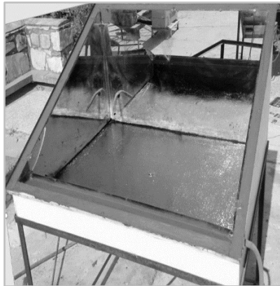
Figure 2(a): A photo to show internal reflector
